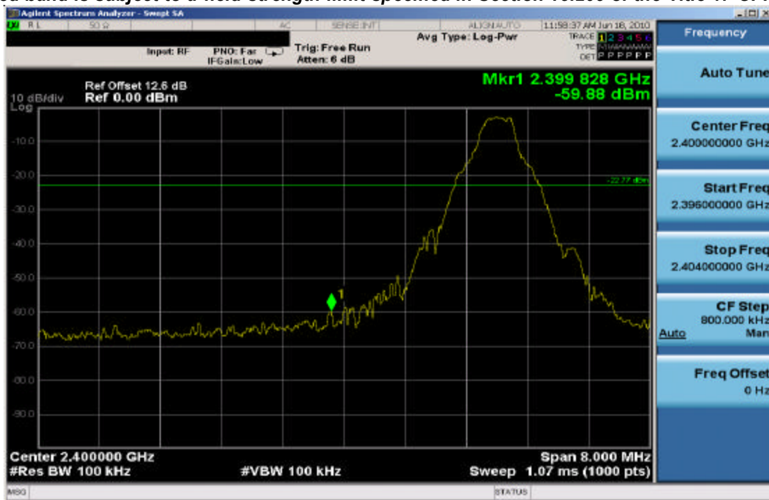
Plot 6-4. Band Edge Plot (Bluetooth – Ch. 0)
