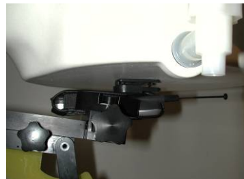
Figure 10-4 Body SAR Sample Photo (Not Actual EUT)
