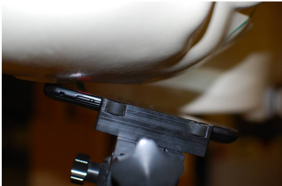
SAR Test Setup Photo 2 – Right Tilt
