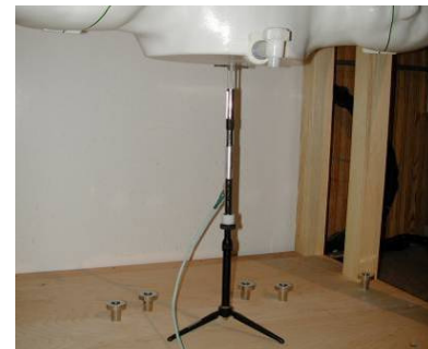
Figure 15-2 System Verification Sample Setup
