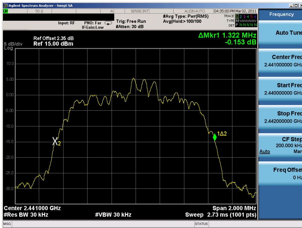
Plot 6-5. 20dB Bandwidth Plot (Bluetooth, 2Mbps – Ch. 39)
