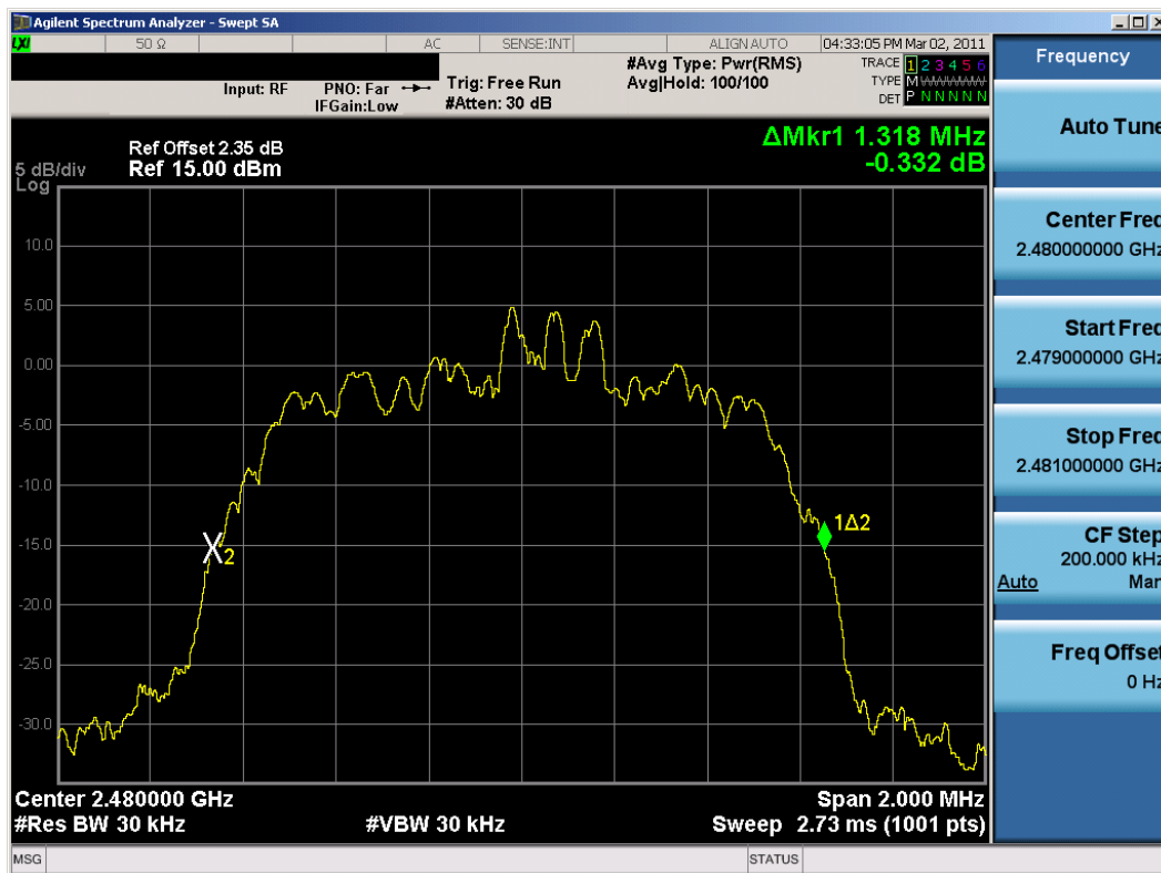
Plot 6-6. 20dB Bandwidth Plot (Bluetooth, 2Mbps – Ch. 78)
