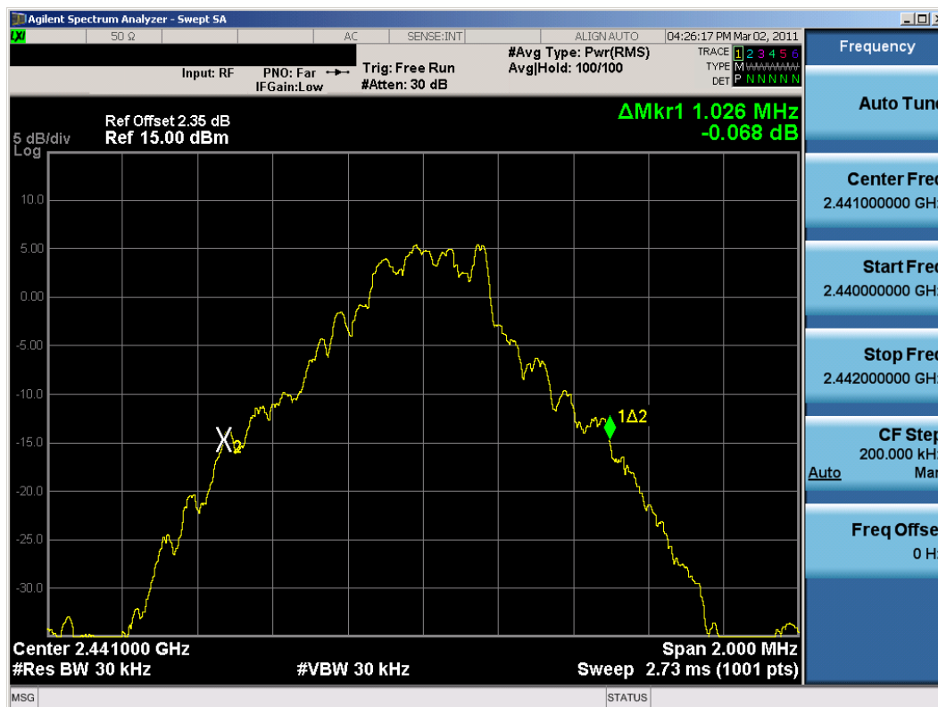
Plot 6-2. 20dB Bandwidth Plot (Bluetooth, 1Mbps – Ch. 39)
