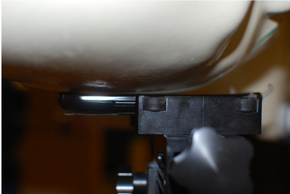
Figure 24-1 SAR Test Setup Photo – Right Touch
