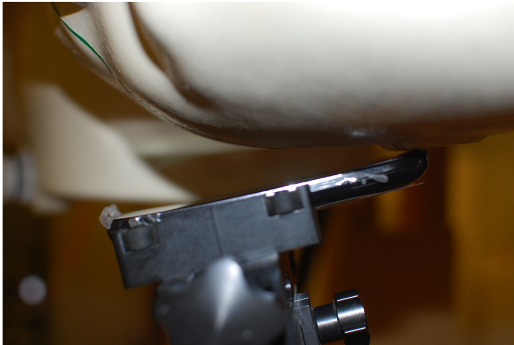
Figure 24-4 SAR Test Setup Photo – Left Tilt
