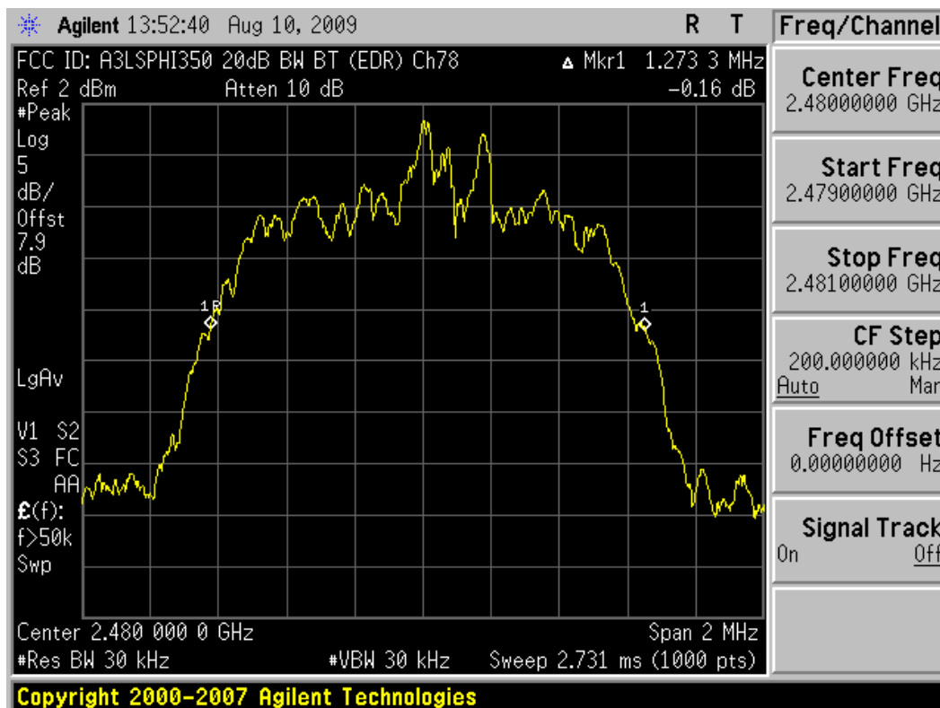
Plot 6-3. 20dB Bandwidth Plot (Bluetooth 2.0 with Enhanced Data Rates – Ch. 78)
