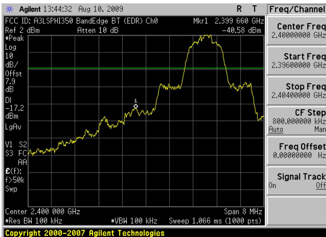
Plot 6-6. Band Edge Plot (Bluetooth 2.0 with Enhanced Data Rates – Ch. 0)
