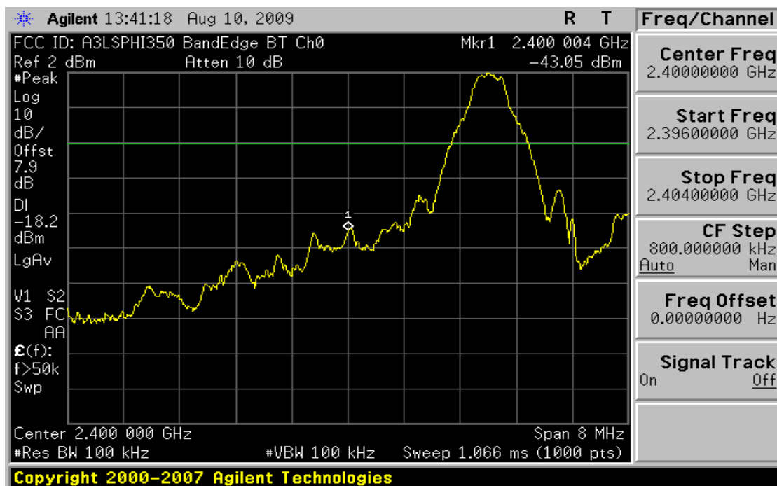
Plot 6-4. Band Edge Plot (Bluetooth – Ch. 0)
