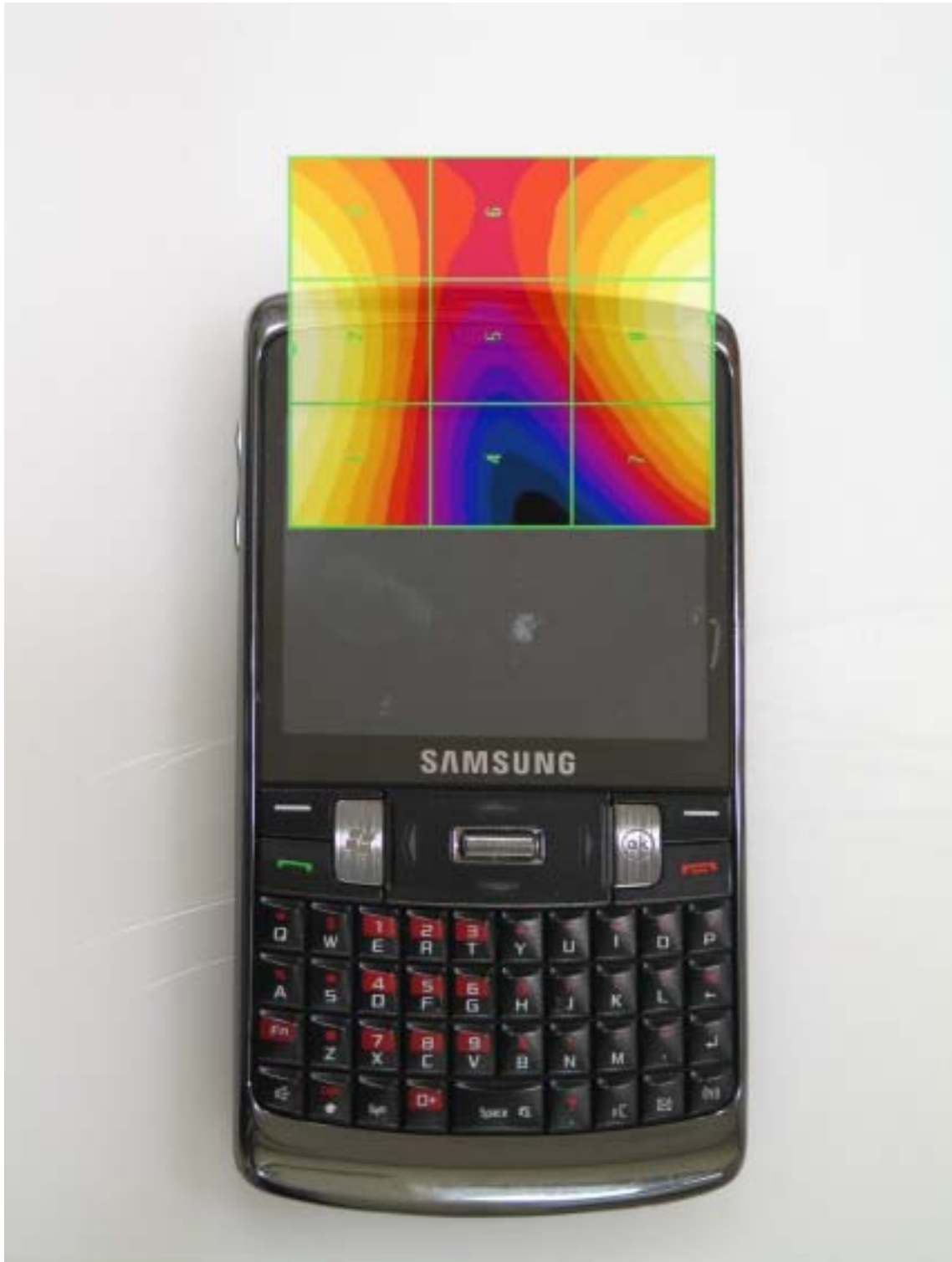
Scan overlay with actual device for CDMA (E-field)
