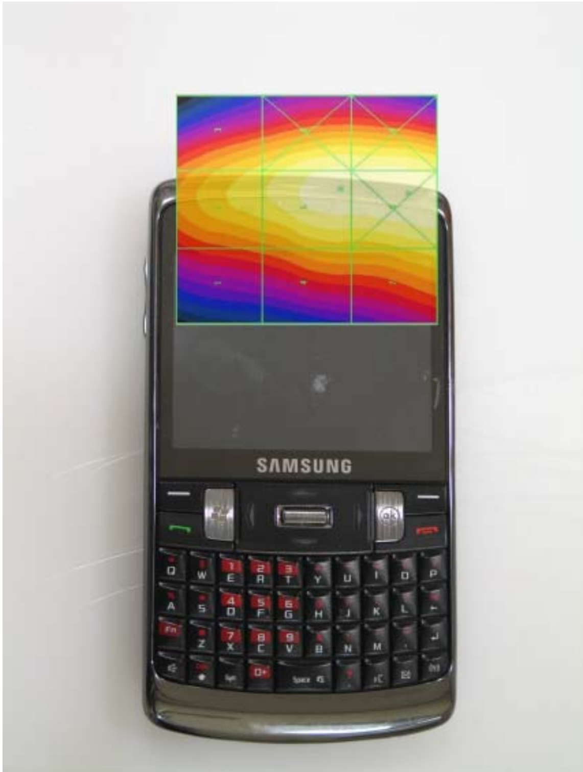
Scan overlay with actual device for GSM (E-field)
