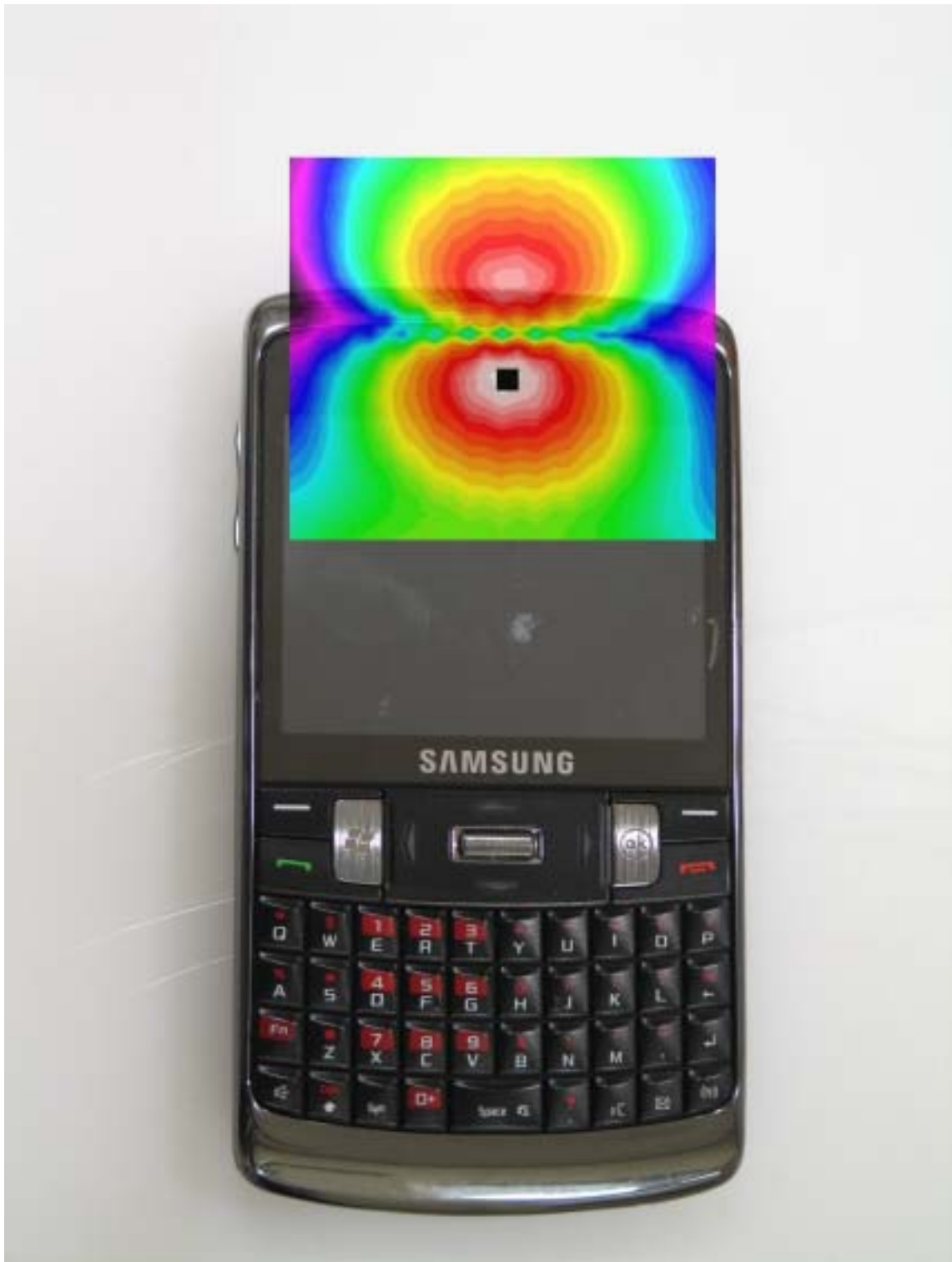
Scan overlay with actual device for GSM (Radial Longitudinal)
