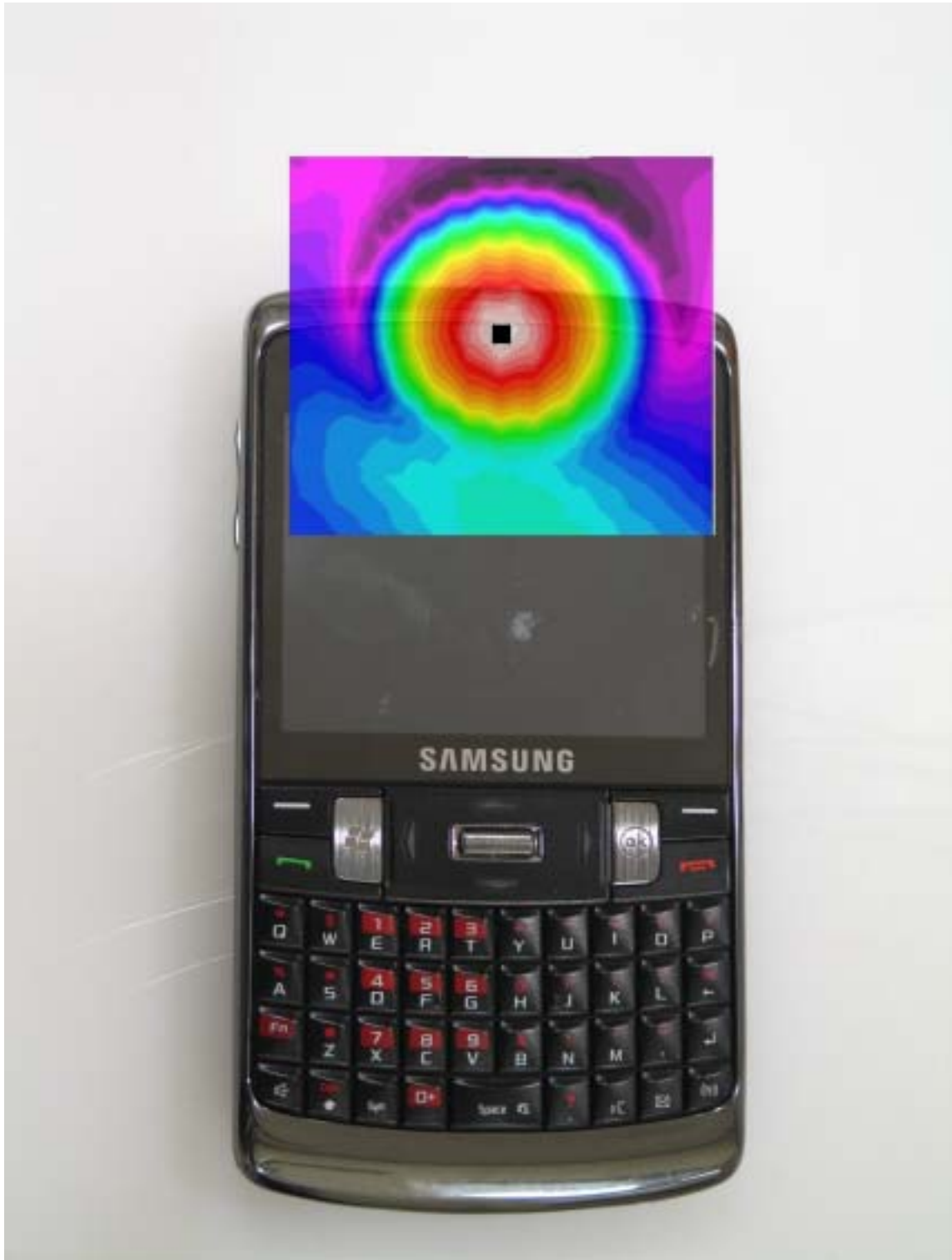
Scan overlay with actual device for GSM (Axial)
