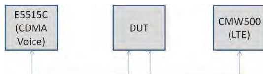
Figure 10-1 SVLTE Conducted Test Setup Diagram
