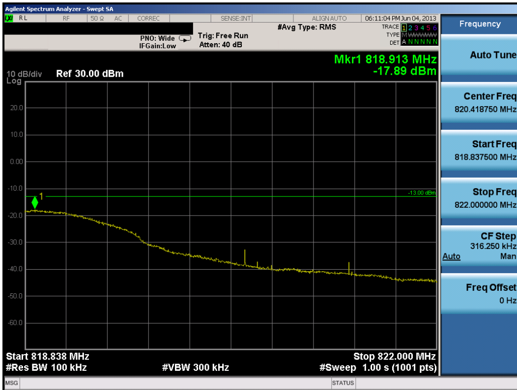
Plot 7-4. Inner Extended Band Edge Plot (Ch. 476)
