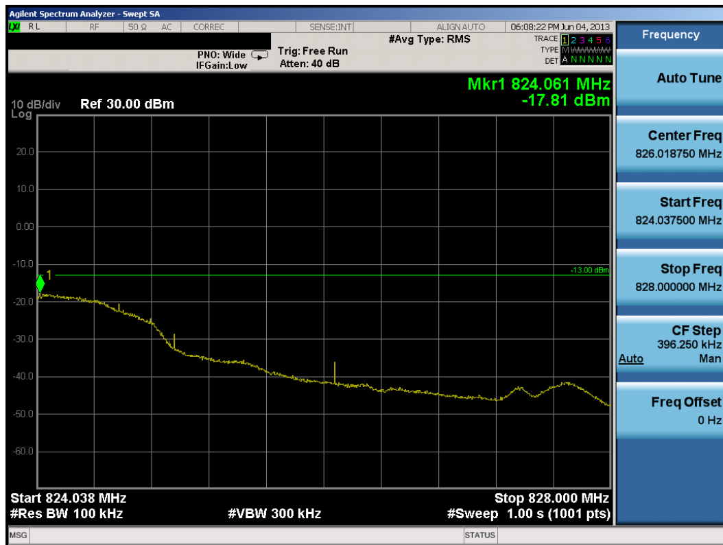
Plot 7-10. Outer Extended Band Edge Plot (Ch. 684)
