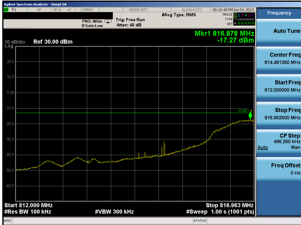
Plot 7-5. Outer Extended Band Edge Plot (Ch. 476)
