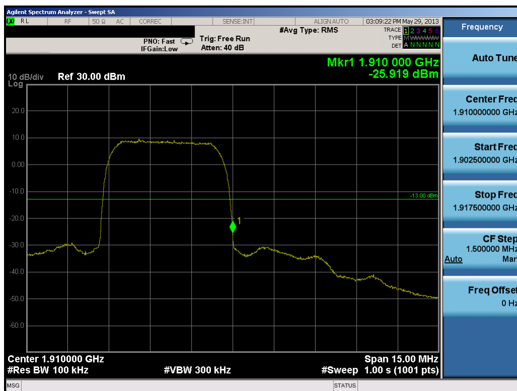
Plot 7-59. Band Edge Plot (PCS WCDMA Mode – Ch. 9538)
