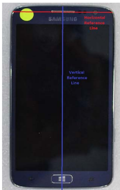
SAR Test Setup Photo 9 - Horizontal and Vertical Reference Lines
