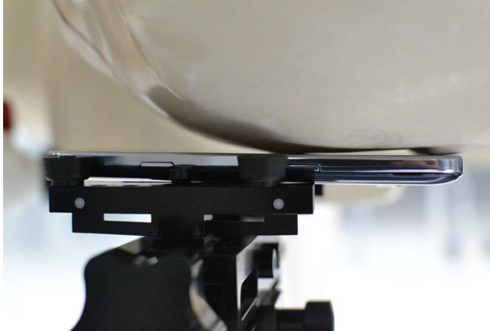
SAR Test Setup Photo 3 - Left Cheek
