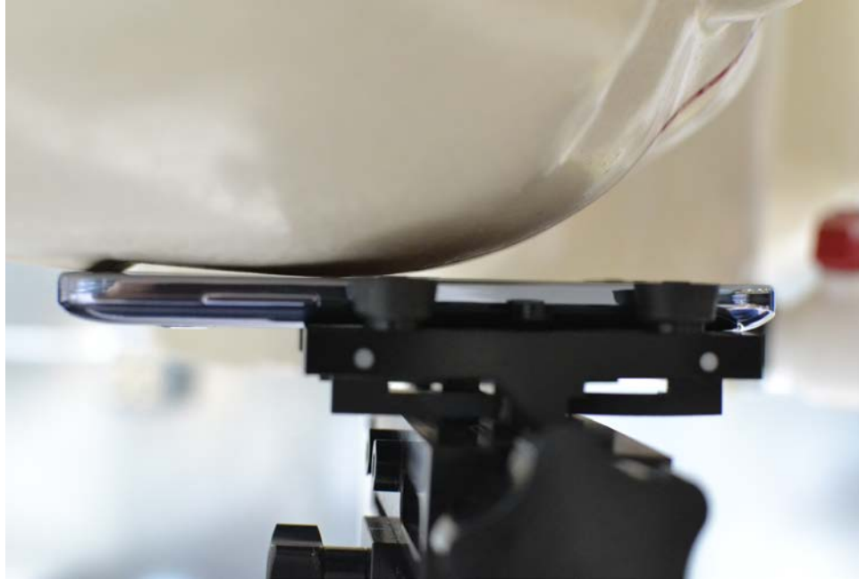
SAR Test Setup Photo 1 - Right Cheek
