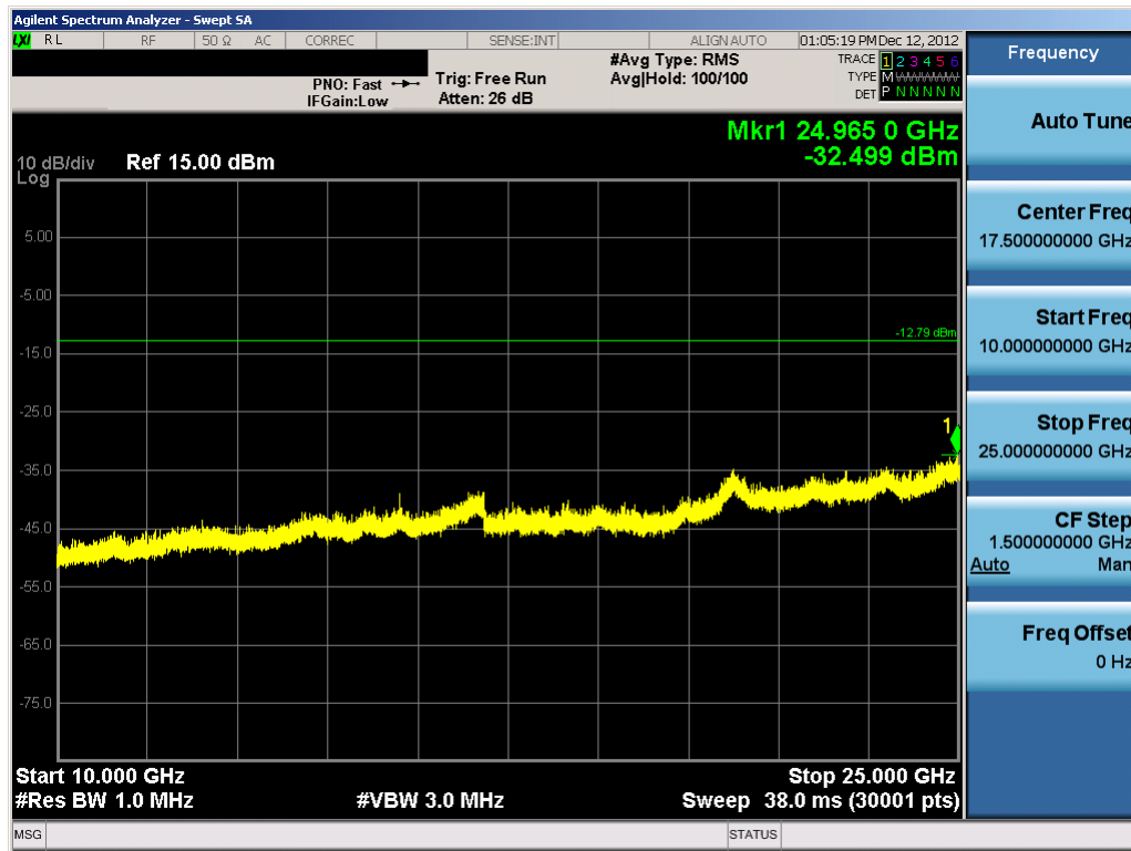
Plot 6-41. Conducted Spurious Plot (Bluetooth, 3Mbps – Ch. 78)
