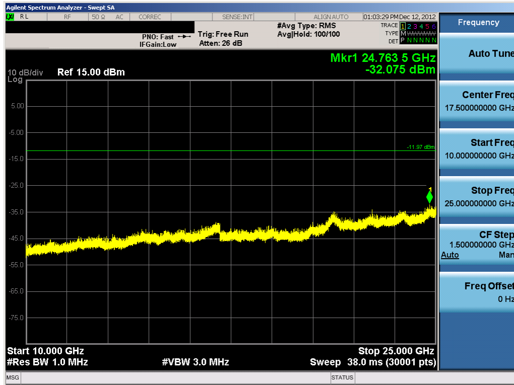
Plot 6-37. Conducted Spurious Plot (Bluetooth, 3Mbps – Ch. 0)
