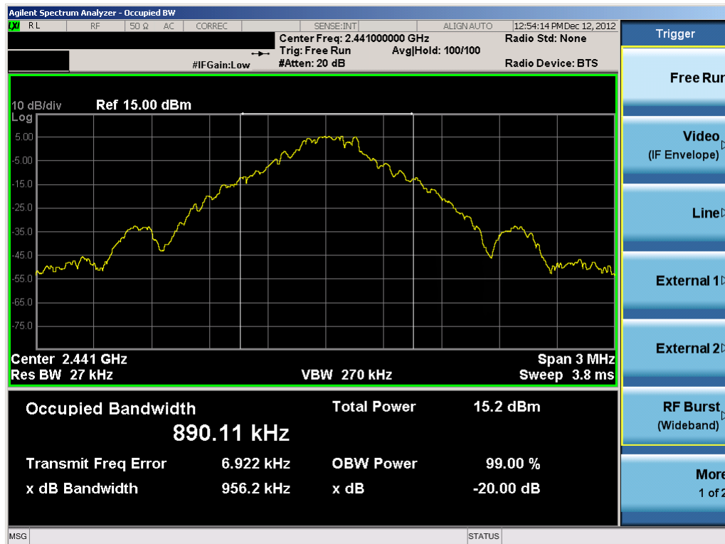
Plot 6-2. 20dB Bandwidth Plot (Bluetooth, 1Mbps – Ch. 39)
