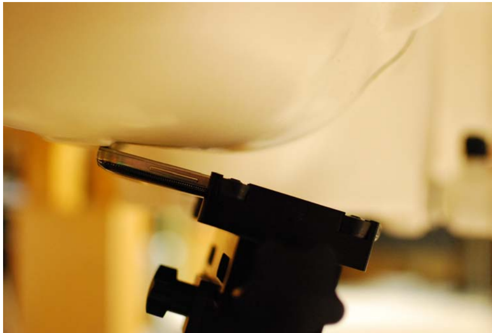
SAR Test Setup Photo 2: Right Tilt
