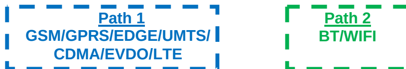
Figure 1-3 Simultaneous Transmission Paths
