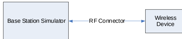
Figure 9-2 Power Measurement Setup
