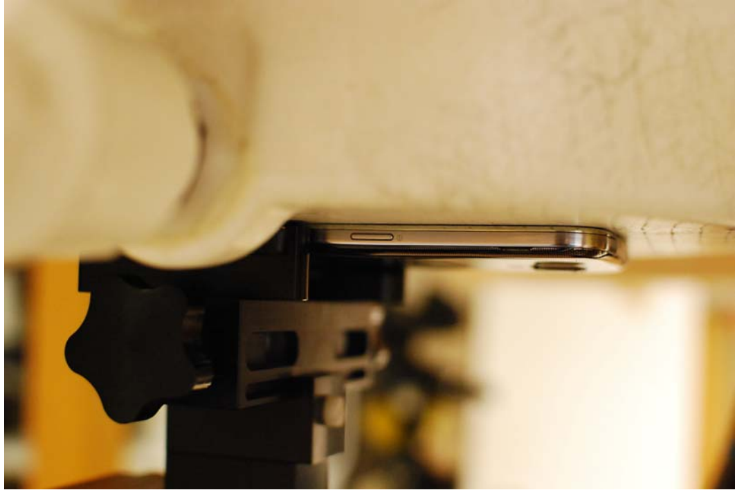
SAR Test Setup Photo 11: Front at 0.0 cm
