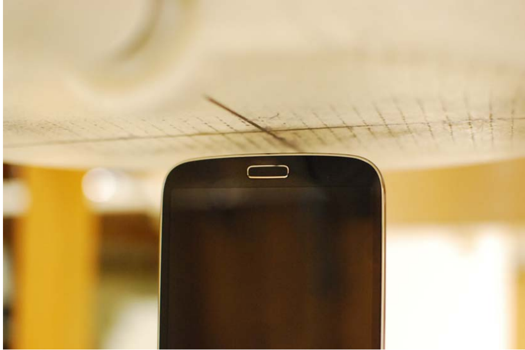
SAR Test Setup Photo 7: Bottom at 1.0 cm
