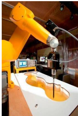
Figure 4-1 SAR Measurement System
