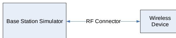
Figure 10-2 Power Measurement Setup
