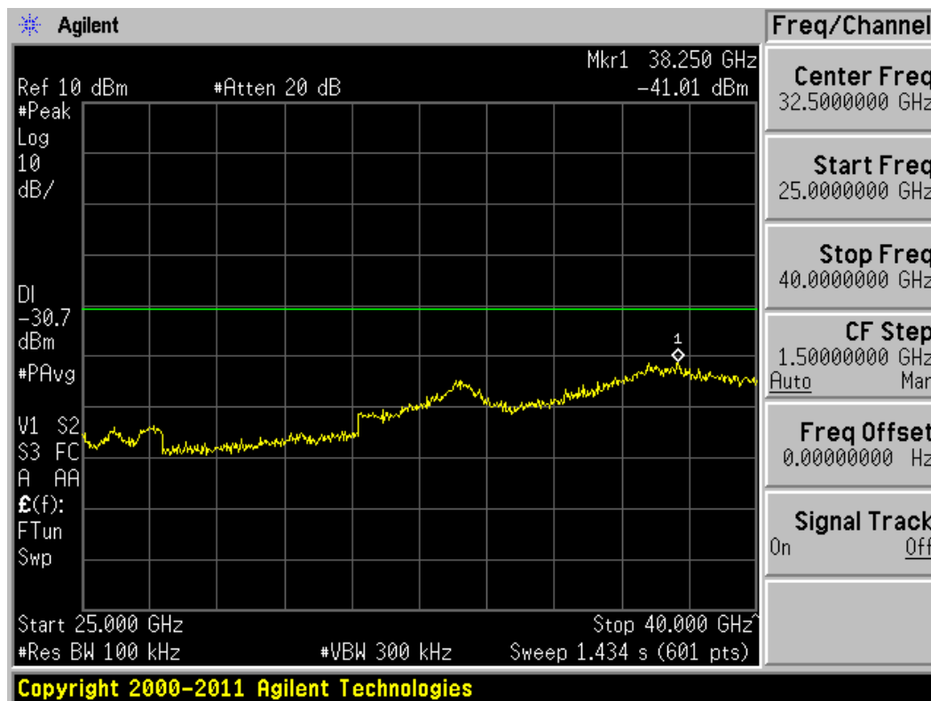
Plot 6-61. Conducted Spurious Plot (802.11a – Ch. 165)
