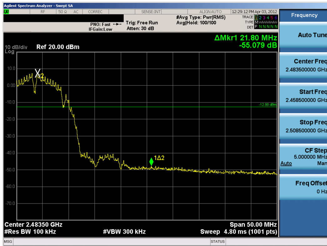
Plot 6-36. Band Edge Plot (802.11b – Ch. 11)
