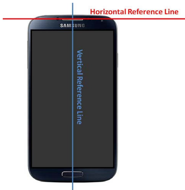
SAR Test Setup Photo 9: DUT Reference Lines
