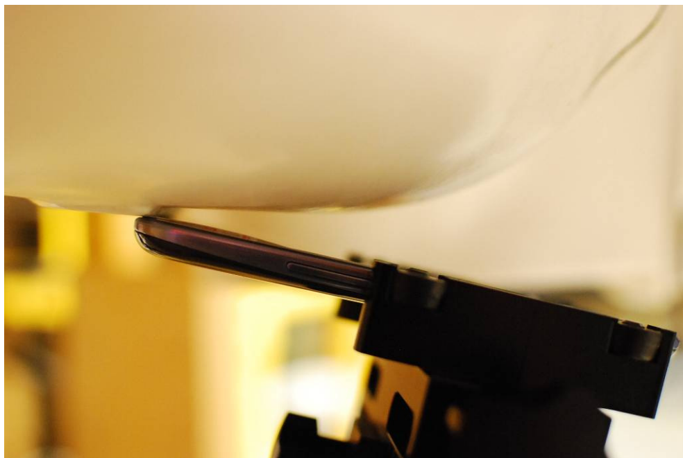
SAR Test Setup Photo 2: Right Tilt
