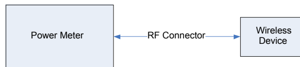
Figure 9-4 Power Measurement Setup
