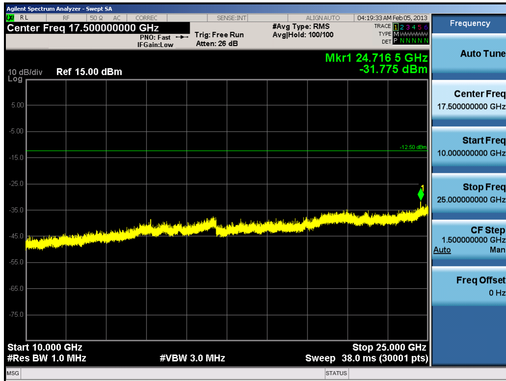
Plot 6-41. Conducted Spurious Plot (Bluetooth, 1Mbps – Ch. 78)
