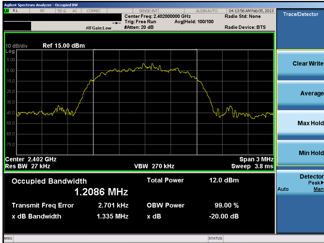
Plot 6-7. 20dB Bandwidth Plot (Bluetooth, 3Mbps – Ch. 0)
