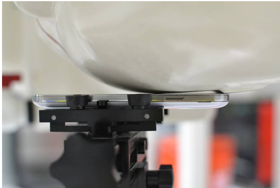
SAR Test Setup Photo 9 - Left Cheek with Wireless Charging Cover
