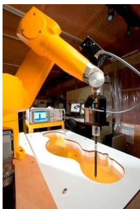
Figure 4-1 SAR Measurement System
