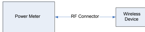
Figure 10-5 Power Measurement Setup
