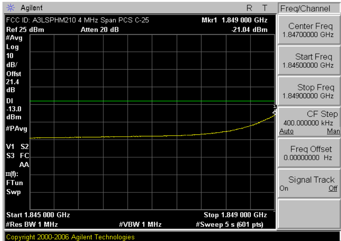
Plot 7-30. 4MHz Span Plot (PCS CDMA Mode – Ch. 25)
