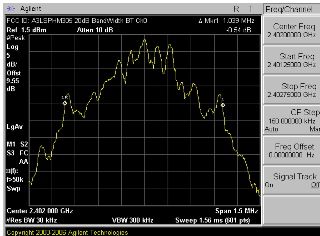
Plot 6-1. 20dB Bandwidth Plot (Bluetooth – Ch. 0)
