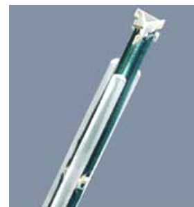
Figure 3.4 Probe Thick-Film Technique
