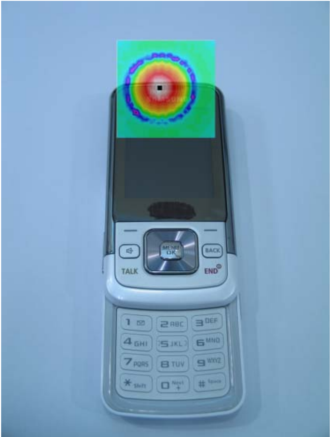
Slide Up Scan overlay with actual device (Axial)
