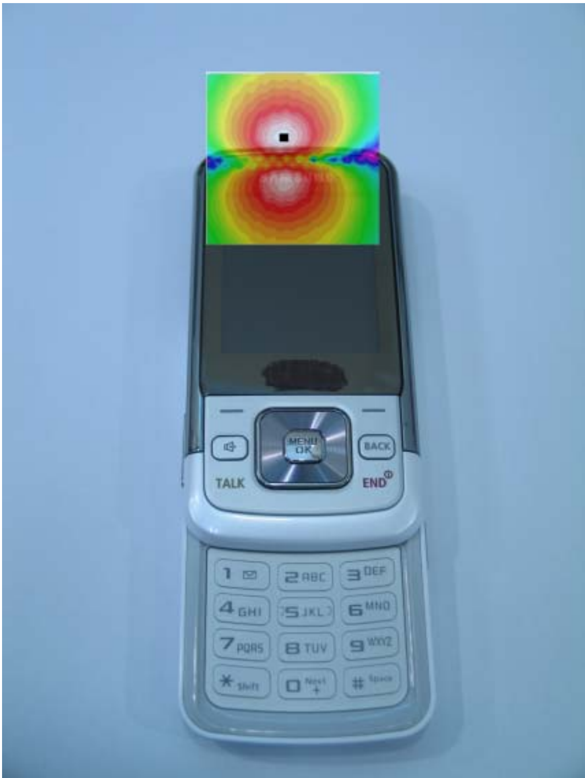
Slide Up Scan overlay with actual device (Radial Longitudinal)
