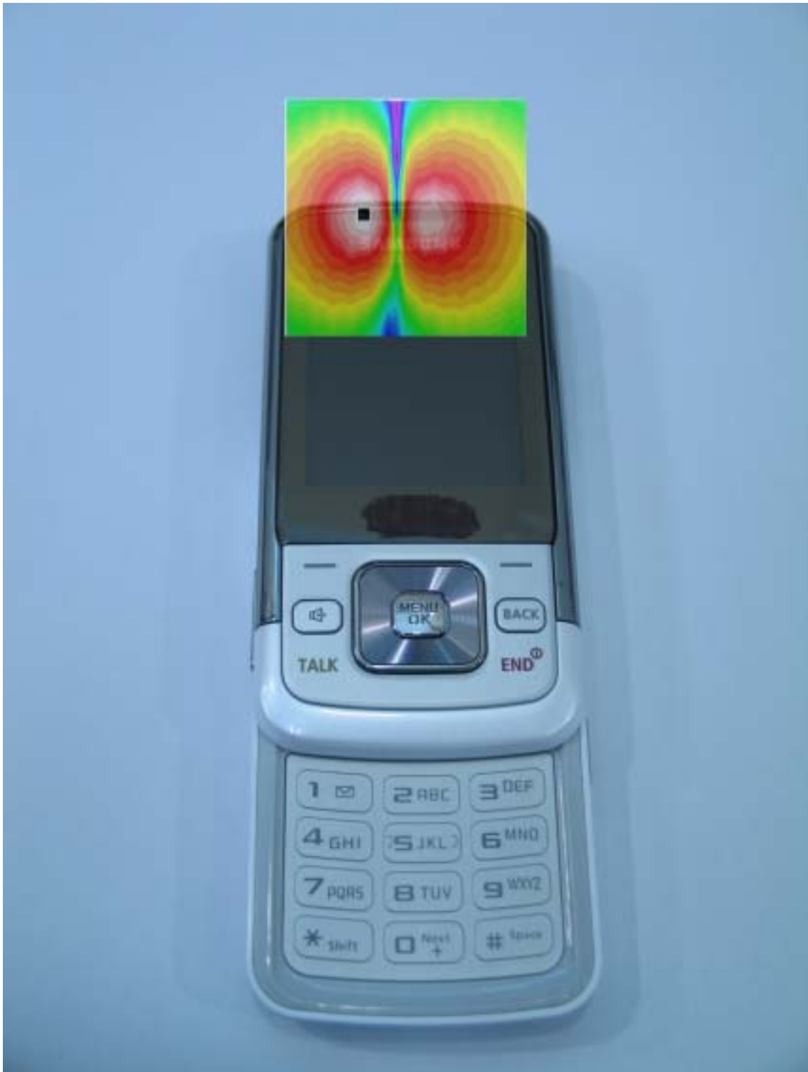
Slide Up Scan overlay with actual device (Radial Transverse)
