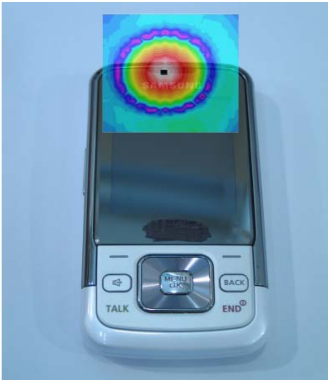
Slide Down Scan overlay with actual device (Axial)
