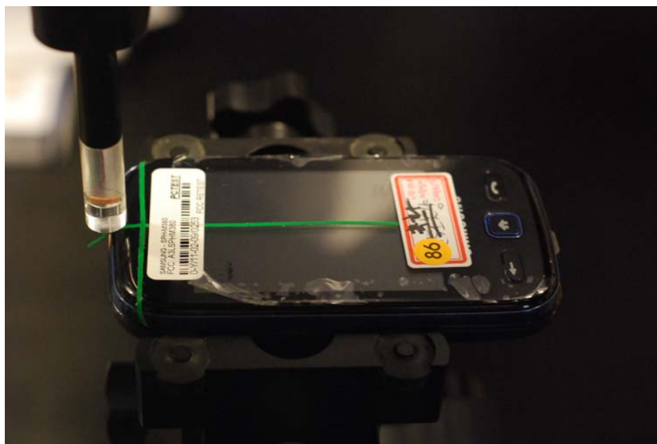
Figure 13-2 Test Setup for Wireless Device
