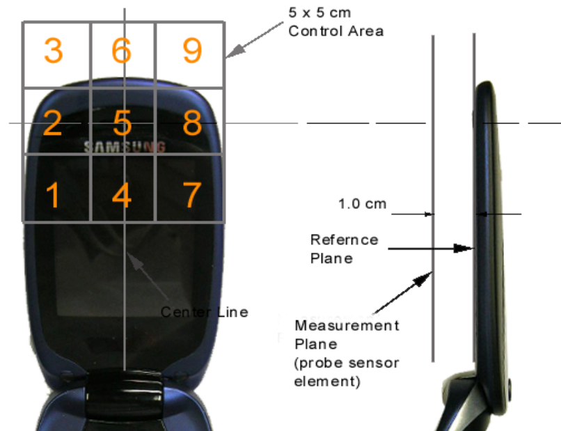
Figure 17-3 5x5 Scan grid above WD
