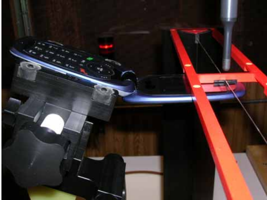
Figure 17-1 Ear Reference Point HAC Phantom Alignment
