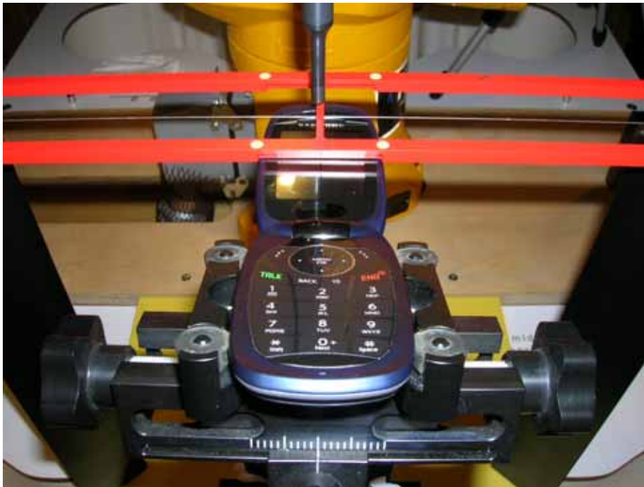
Figure 17-2 HAC Phantom Plane Alignment
