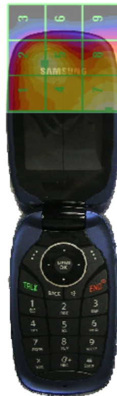
Figure 17-5 H-Field WD Scan overlay
