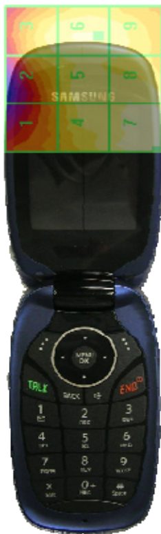
Figure 17-4 E-Field WD Scan overlay
