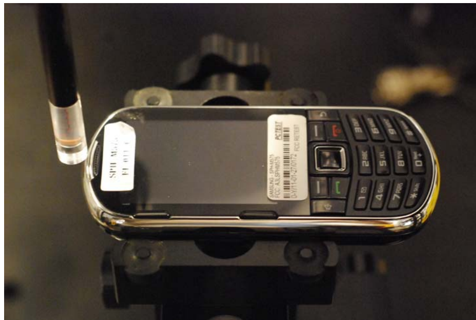
Figure 13-2 Test Setup for Wireless Device
