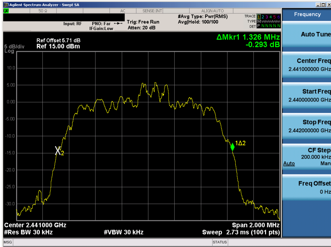
Plot 6-5. 20dB Bandwidth Plot (Bluetooth, 2Mbps – Ch. 39)
