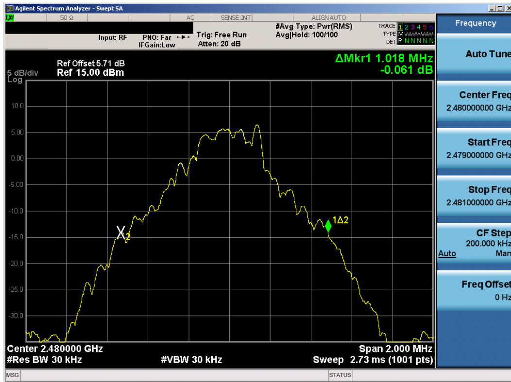
Plot 6-3. 20dB Bandwidth Plot (Bluetooth, 1Mbps – Ch. 78)
