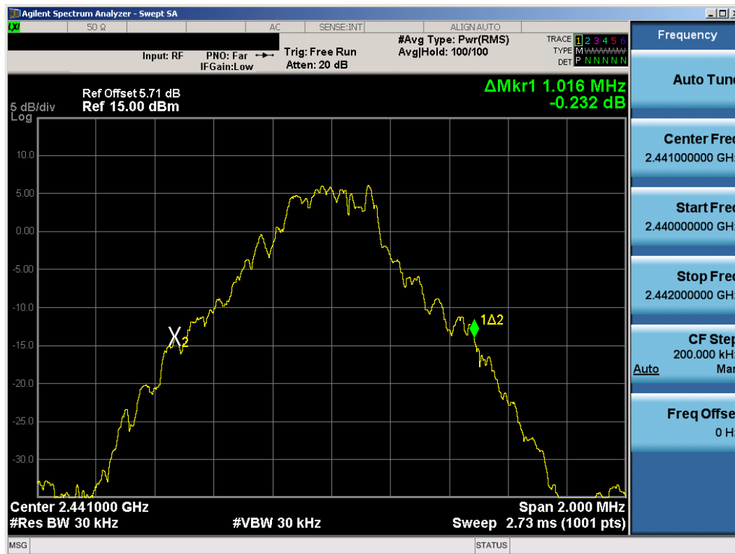
Plot 6-2. 20dB Bandwidth Plot (Bluetooth, 1Mbps - Ch. 39)
