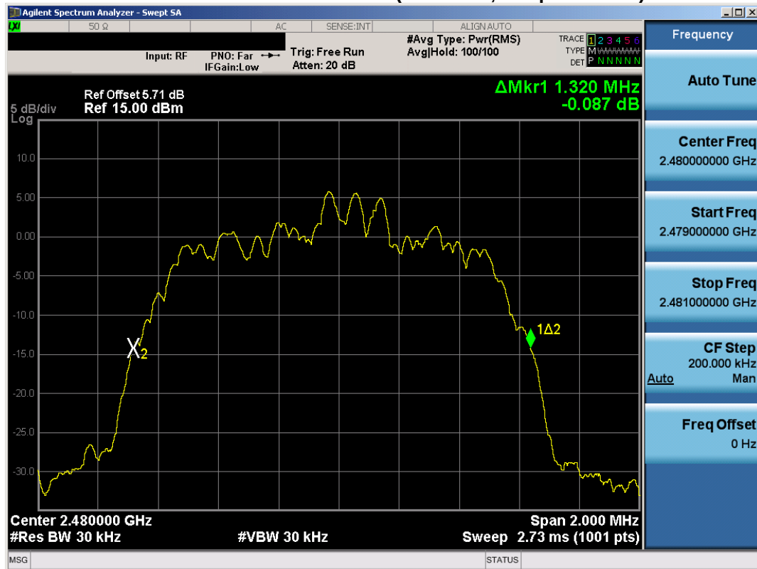
Plot 6-6. 20dB Bandwidth Plot (Bluetooth, 2Mbps – Ch. 78)
