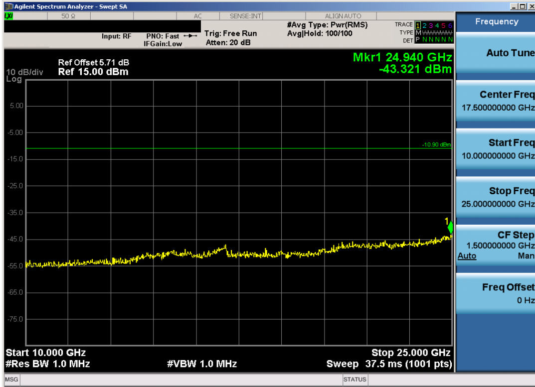
Plot 6-23. Conducted Spurious Plot (Bluetooth, 2Mbps – Ch. 78)
