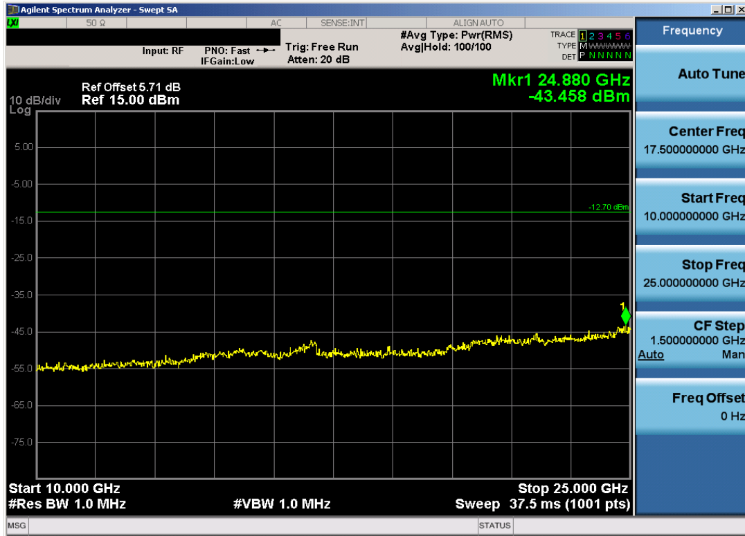
Plot 6-21. Conducted Spurious Plot (Bluetooth, 2Mbps – Ch. 39)
