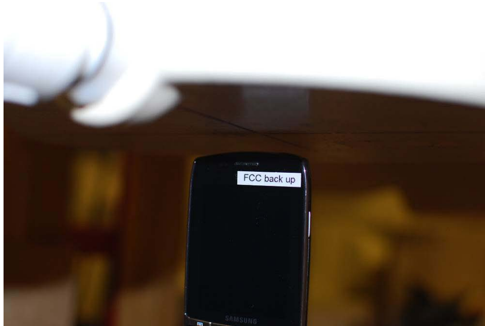
Figure 21-7 SAR Test Setup Photo 7 – Top at 1.0 cm
