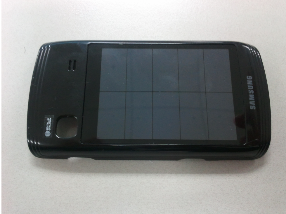
Figure 21-11 SAR Test Setup Photo 10 – Solar Battery Cover
