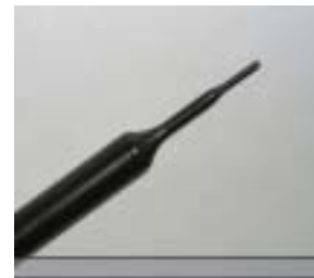
Figure 3.4 Probe Thick-Film Technique
