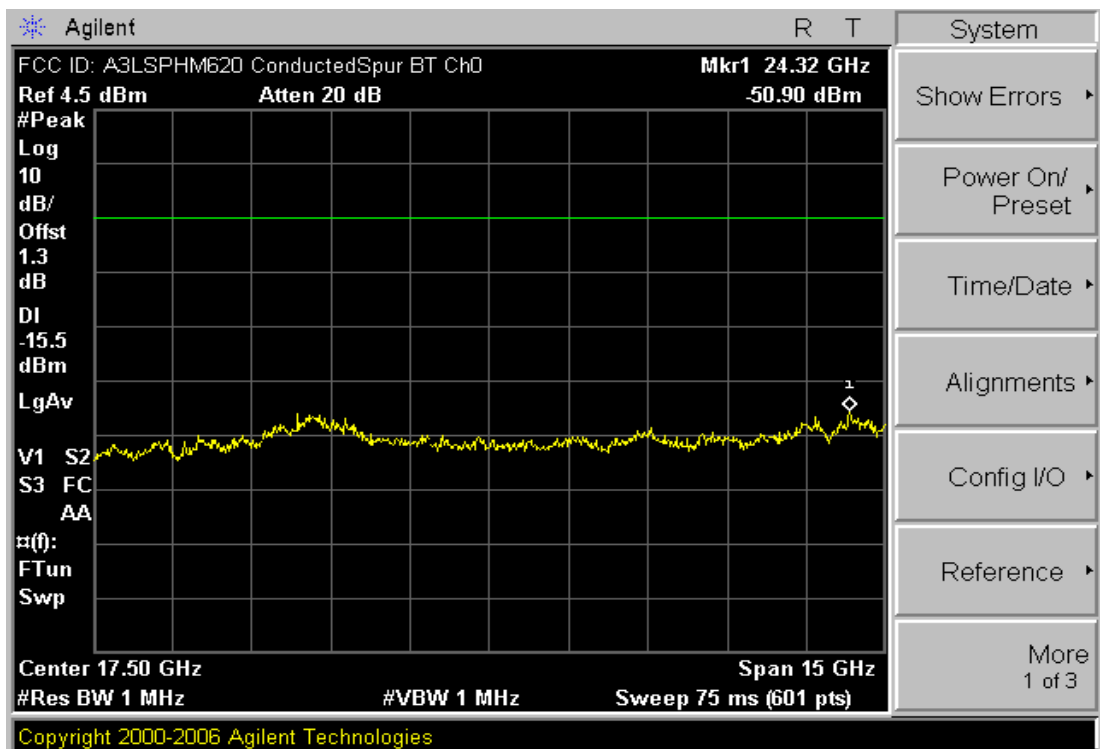
Plot 6-13. Conducted Spurious Plot (Bluetooth – Ch. 0)
