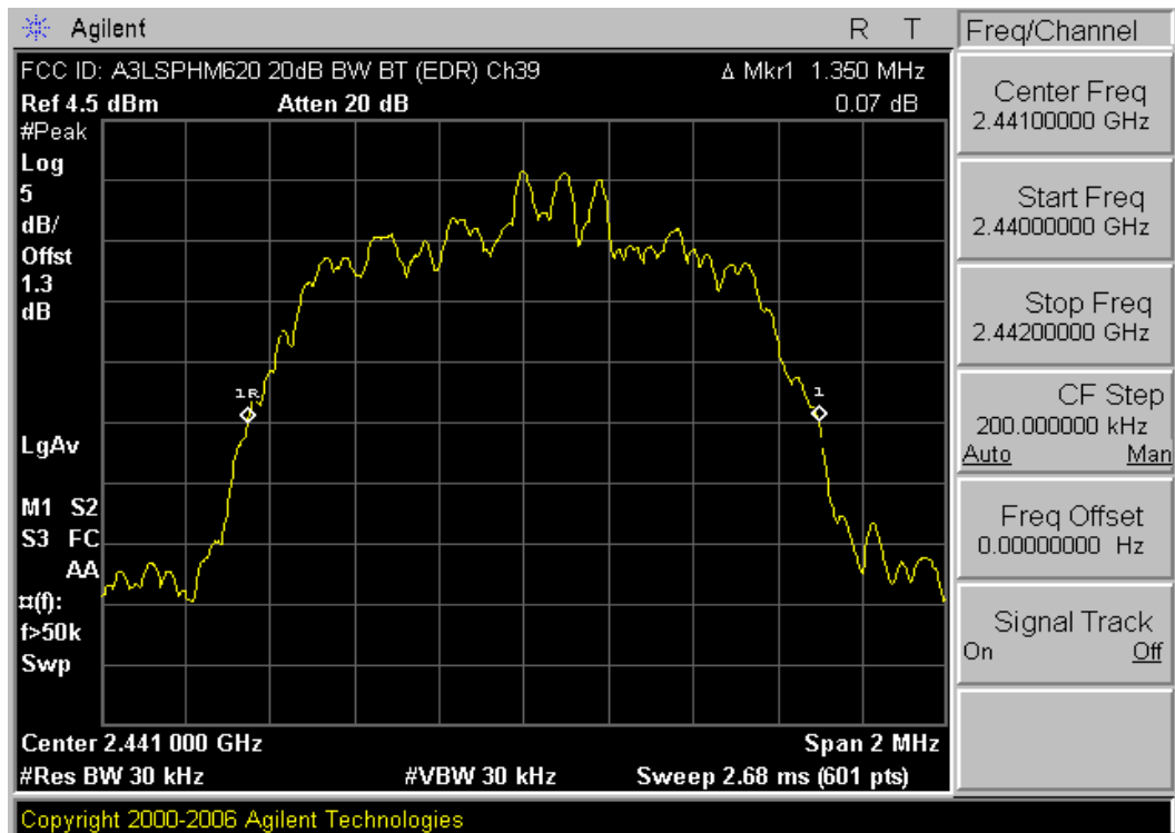
Plot 6-2. 20dB Bandwidth Plot (Bluetooth 2.0 with Enhanced Data Rate – Ch. 39)
