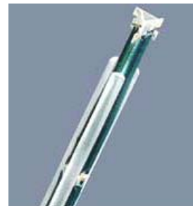
Figure 3.4 Probe Thick-Film Technique
