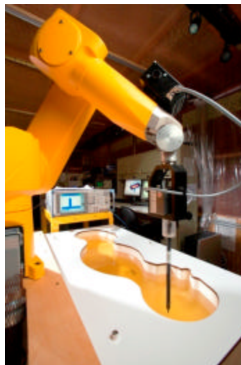
Figure 3-2 DASY4 SAR Measurement System
