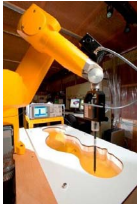
Figure 3-1 SAR Measurement System
