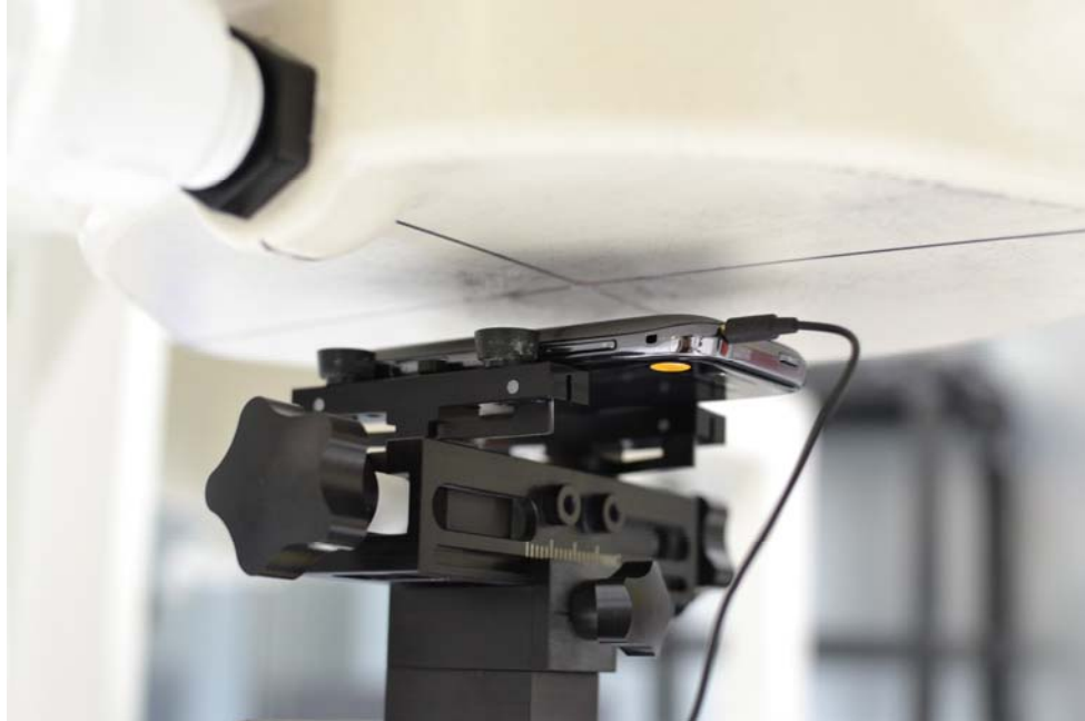
SAR Test Setup Photo 5: Body-worn at 1.5 cm
