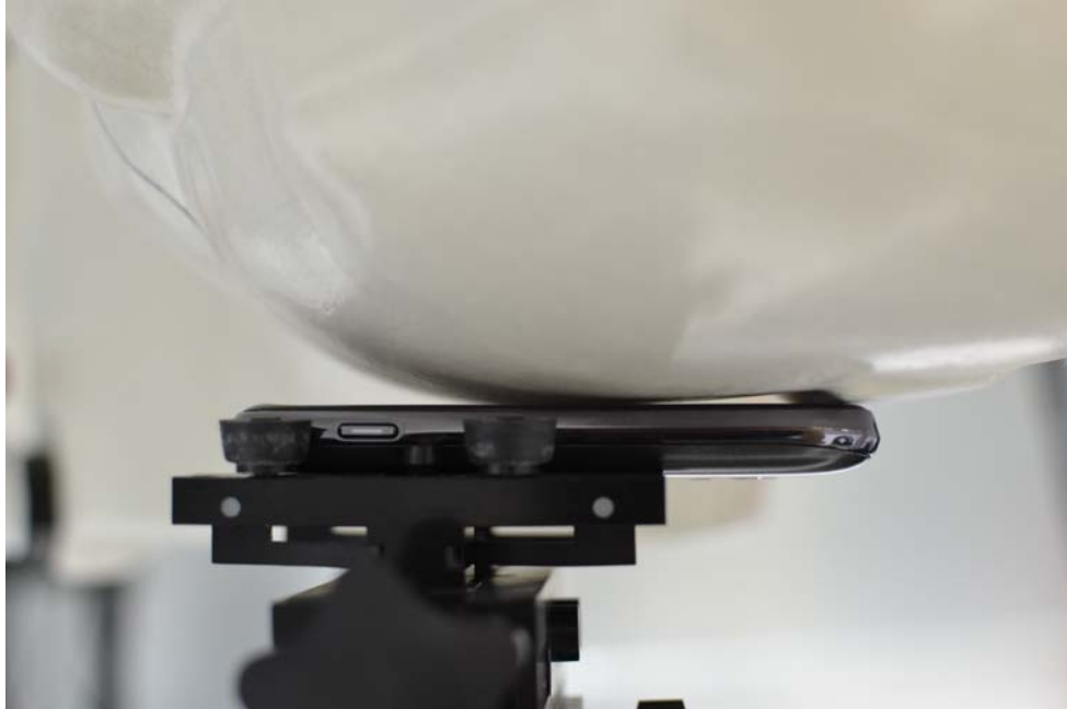
SAR Test Setup Photo 3: Left Touch
