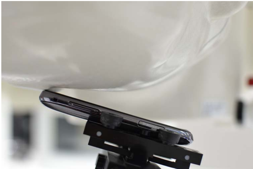
SAR Test Setup Photo 2: Right Tilt
