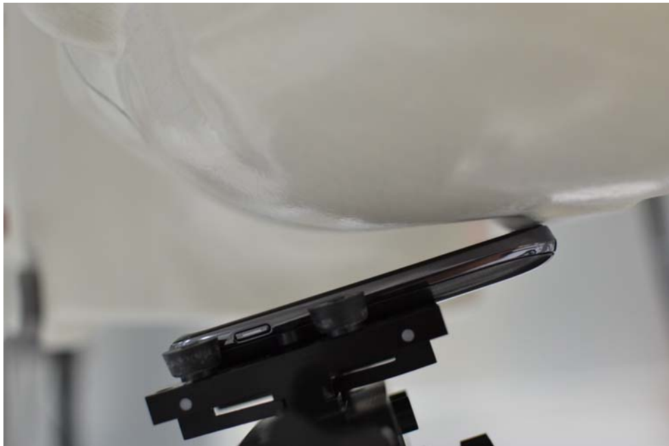
SAR Test Setup Photo 4: Left Tilt
