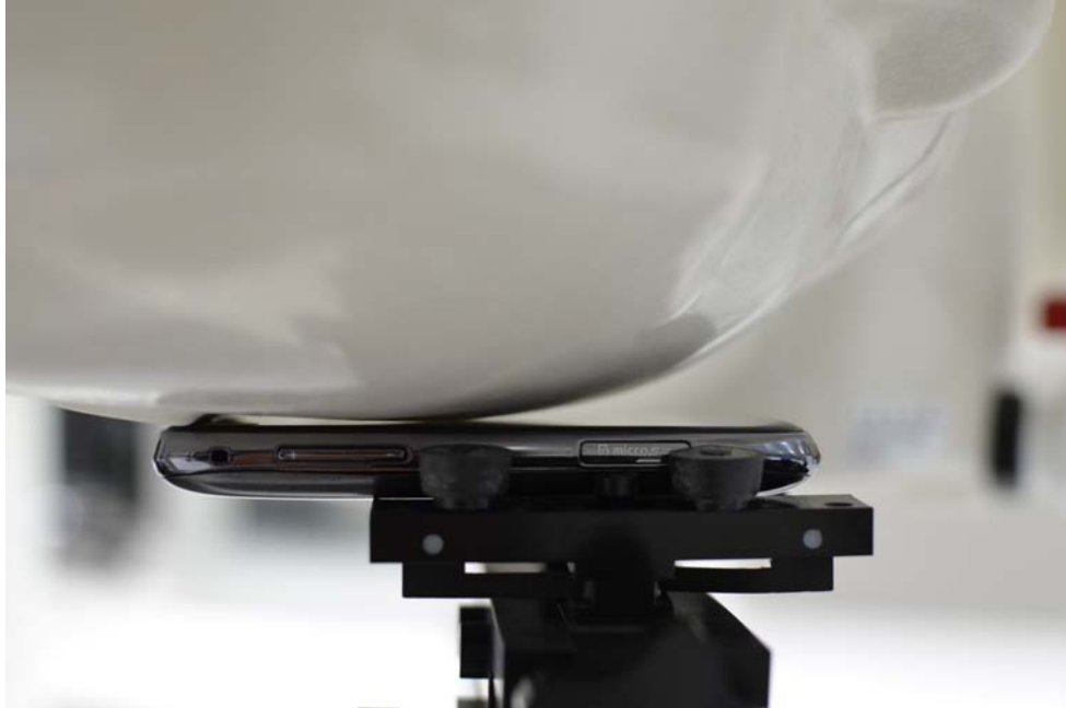
SAR Test Setup Photo 1: Right Touch
