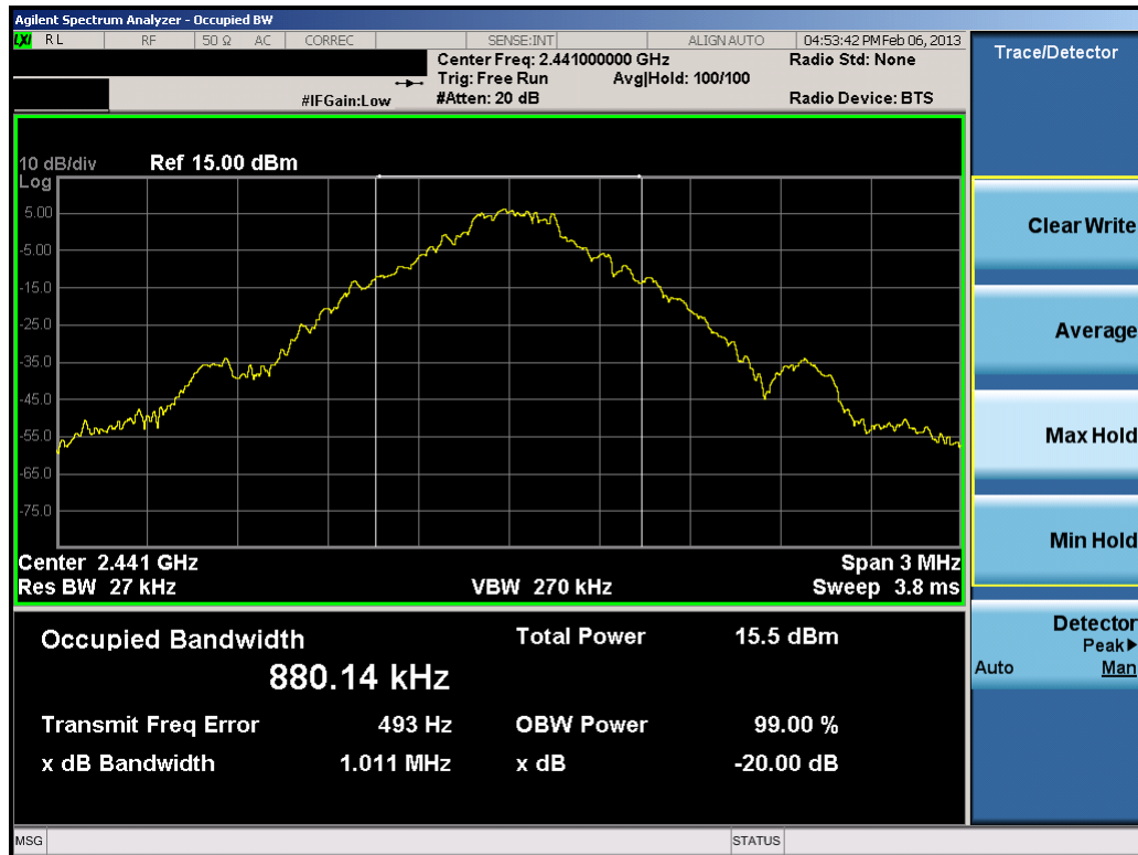
Plot 6-2. 20dB Bandwidth Plot (Bluetooth, 1Mbps – Ch. 39)
