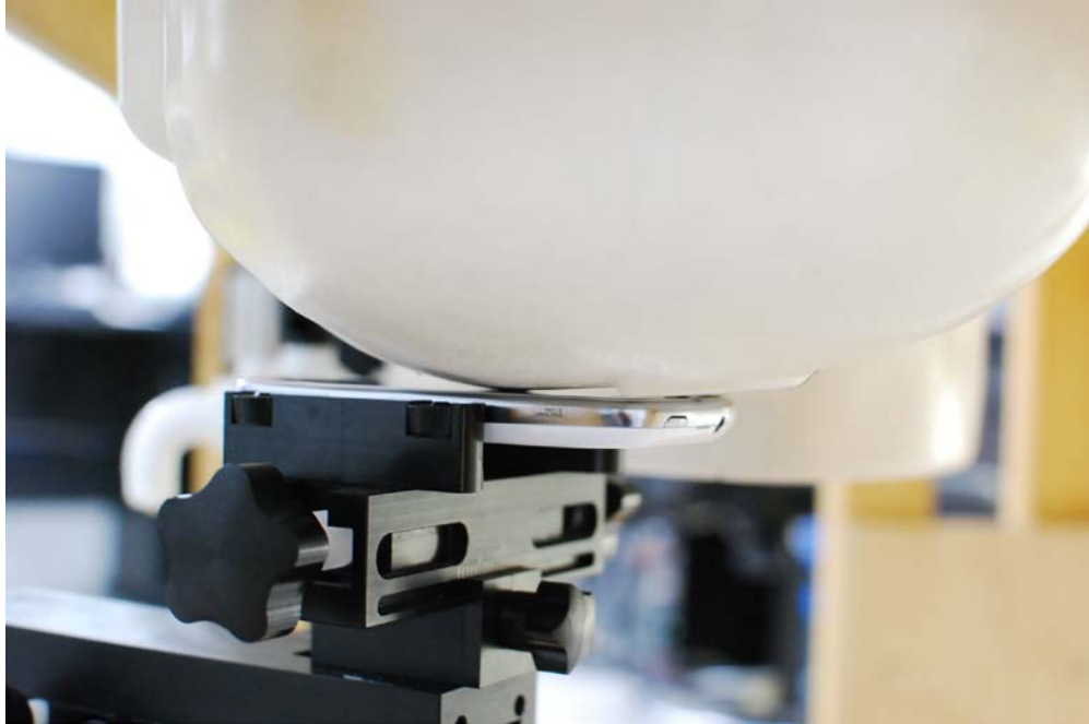
SAR Test Setup Photo 1: Left Cheek
