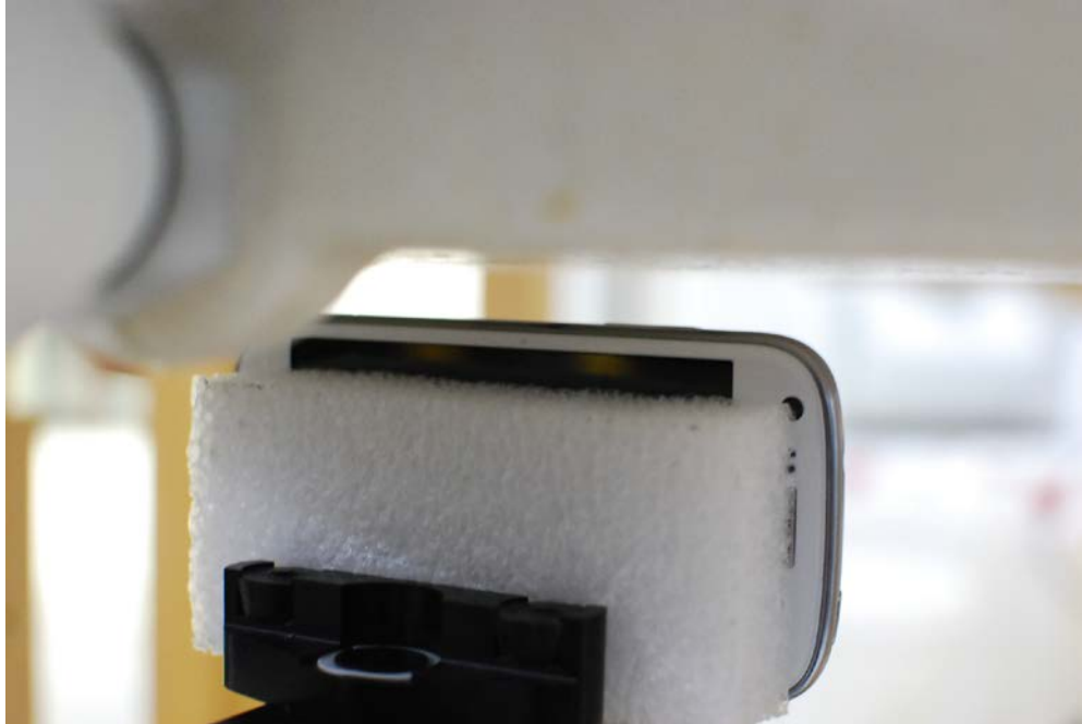
SAR Test Setup Photo 7: Left Edge at 1.0 cm
