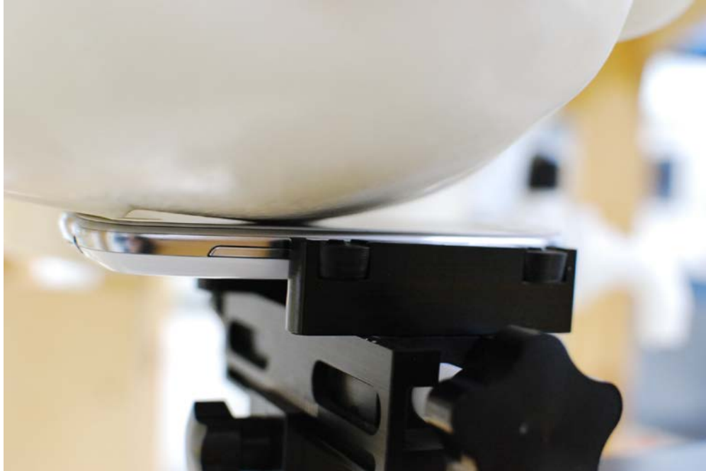
SAR Test Setup Photo 3: Right Cheek
