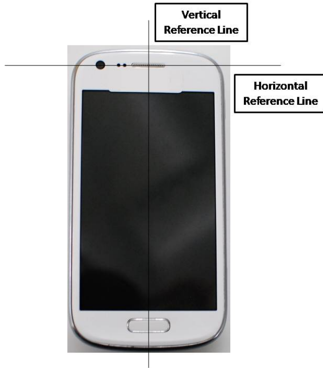
SAR Test Setup Photo 11: Vertical and Horizontal Reference Lines
