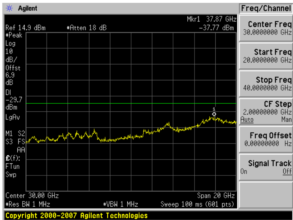
Plot 6-50. Conducted Spurious Plot (802.11a – Ch. 157)
