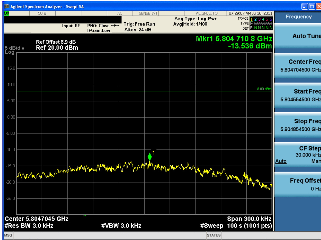
Plot 6-24. Power Spectral Density Plot (802.11a – Ch. 161)
