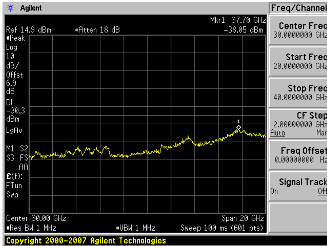
Plot 6-48. Conducted Spurious Plot (802.11a – Ch. 149)
