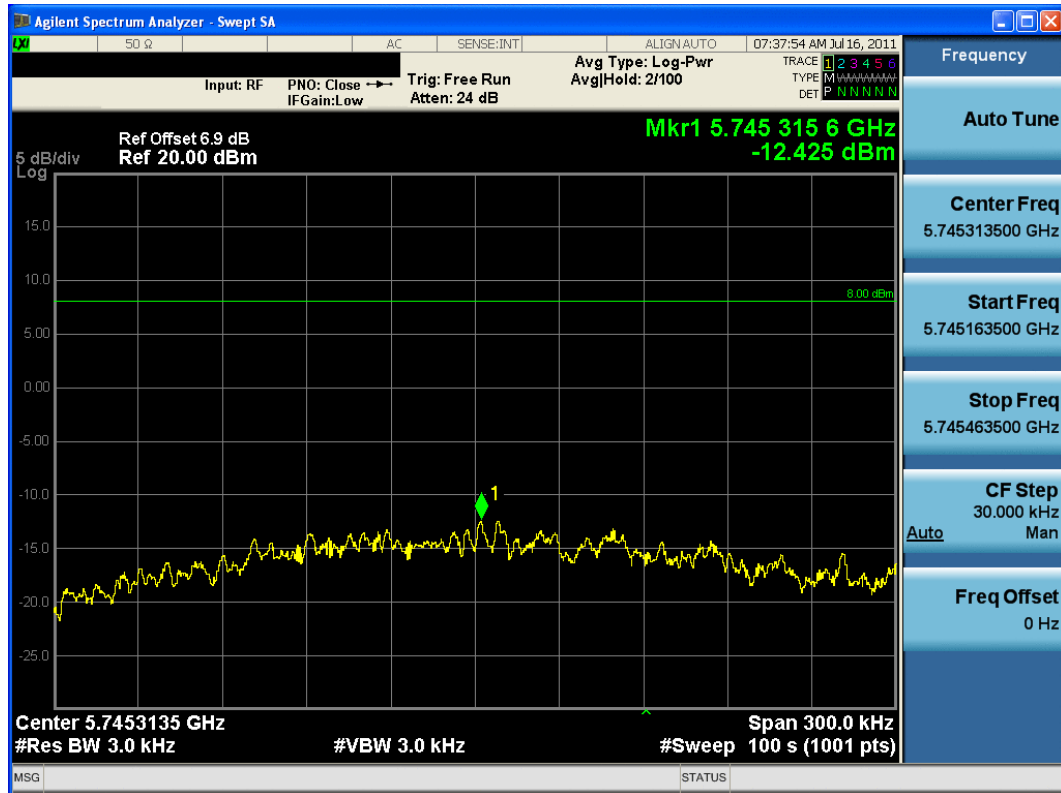
Plot 6-22. Power Spectral Density Plot (802.11a – Ch. 149)
