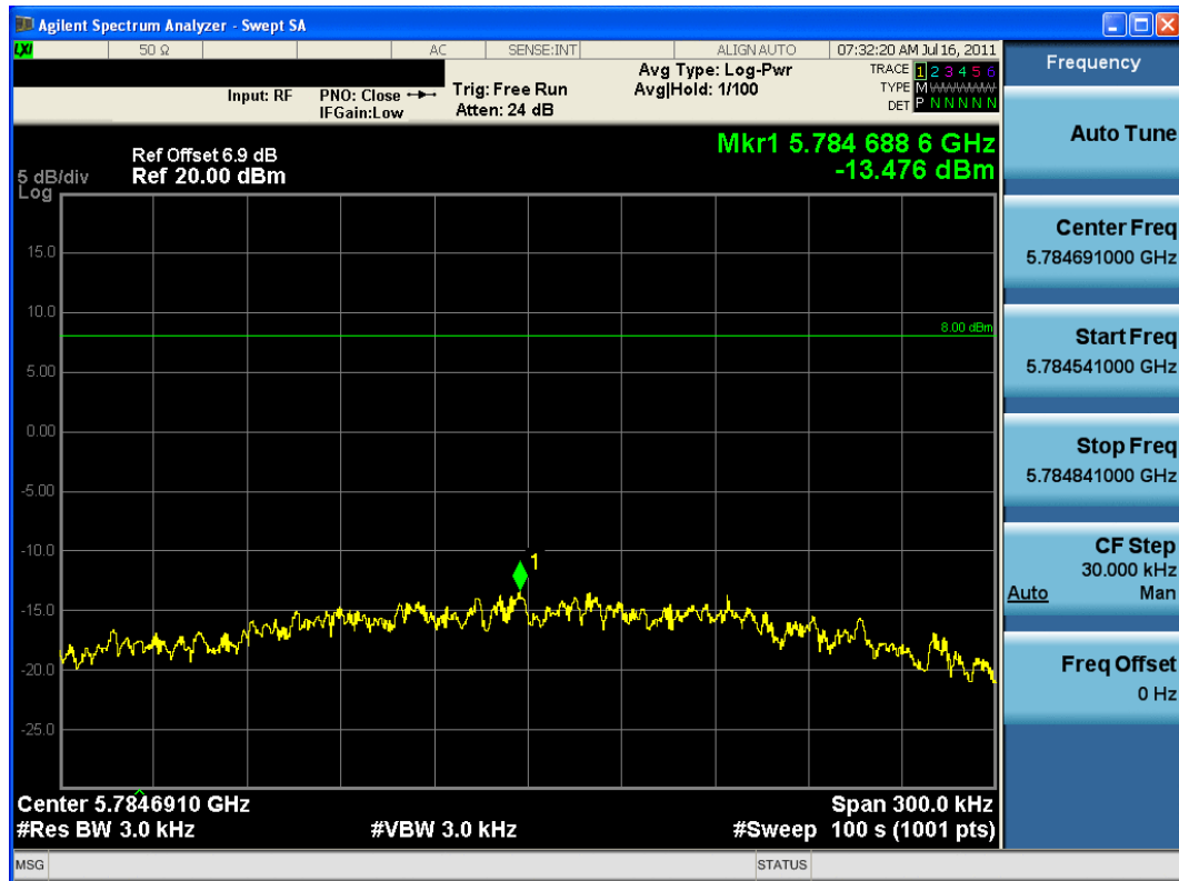
Plot 6-23. Power Spectral Density Plot (802.11a – Ch. 157)
