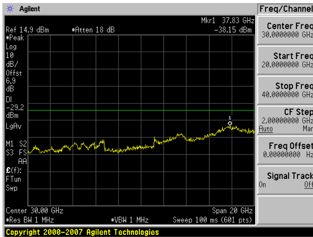
Plot 6-52. Conducted Spurious Plot (802.11a – Ch. 161)
