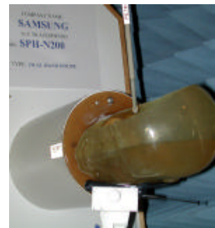
Fig. 1 SAR Test Setup
