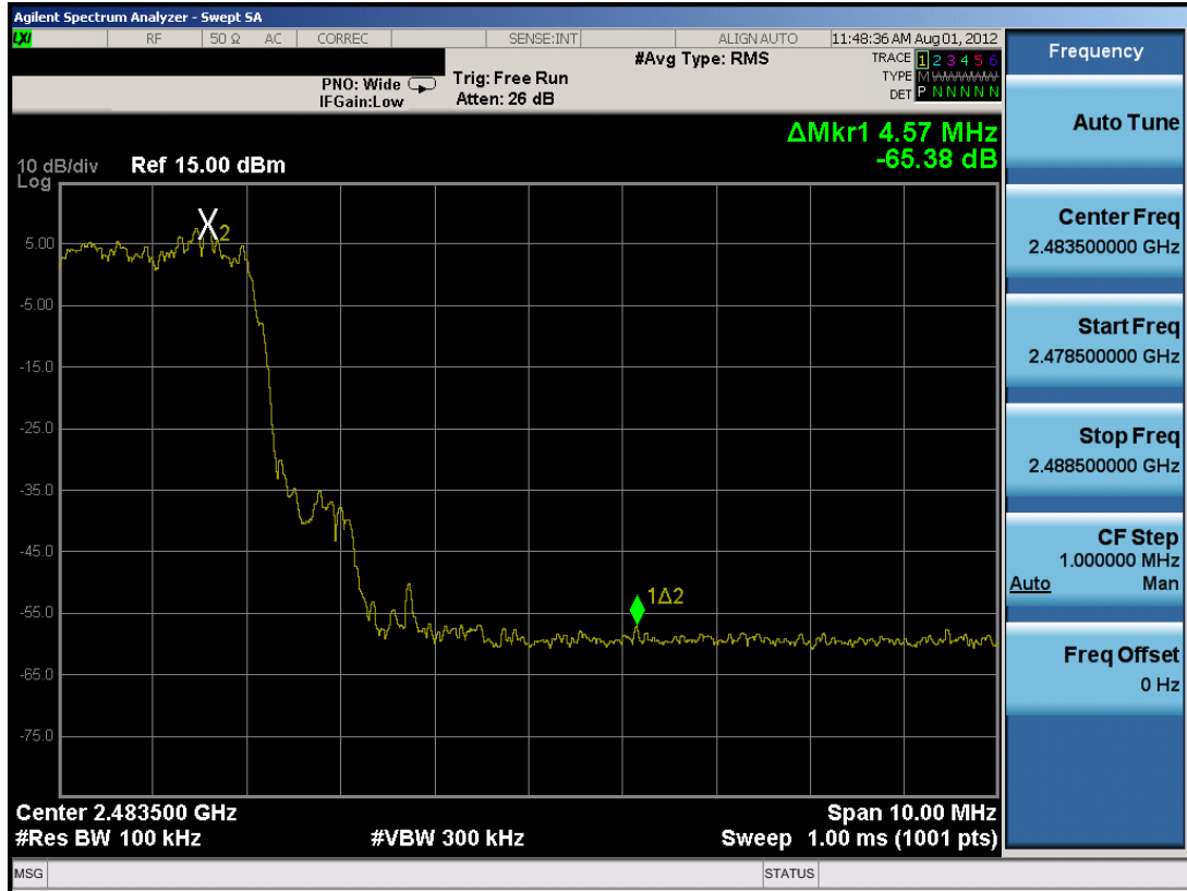
Plot 6-13. Band Edge Plot (Bluetooth with Hopping Enabled, 3Mbps)
