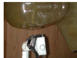
Fig. A Head SAR Test Setup
