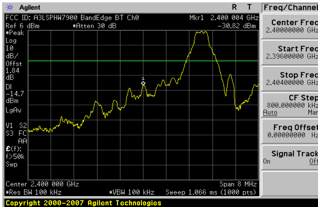
Plot 6-4. Band Edge Plot (Bluetooth – Ch. 0)
