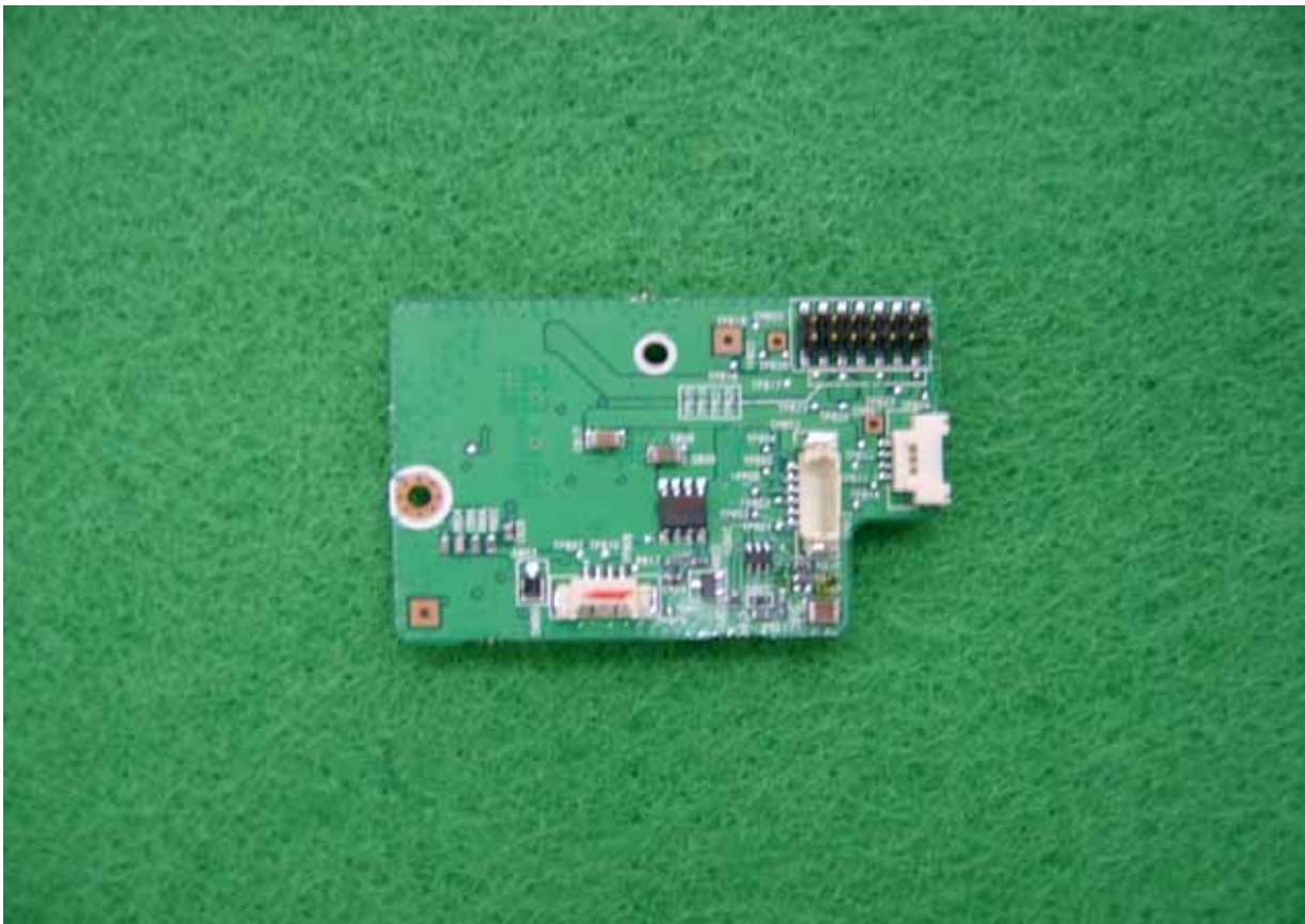
Power board bottom view
