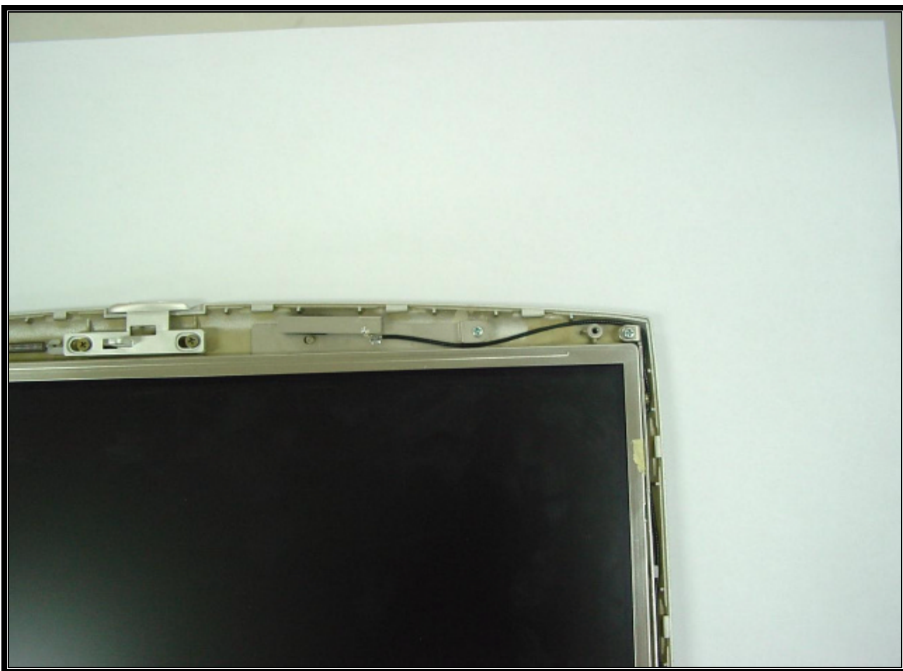
PHOTOGRAPH 10: TOP VIEW OF MAIN TRANSMITTING ANTENNA
